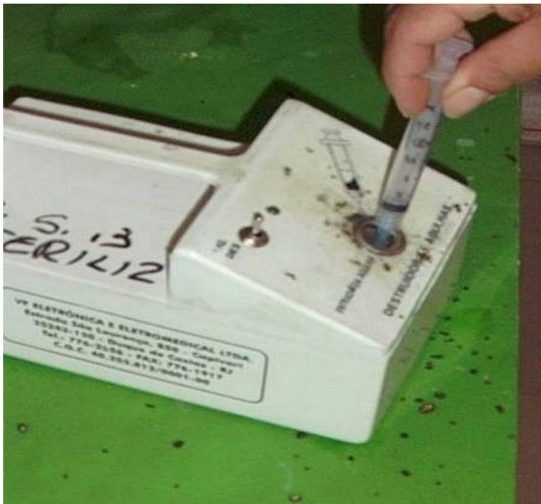
Figure E8. Splatter around inlet hole and adjacent countertop after clinical use of electrical needle destroyer device of Brazilian manufacture (photograph courtesy: Anthony Battersby).
