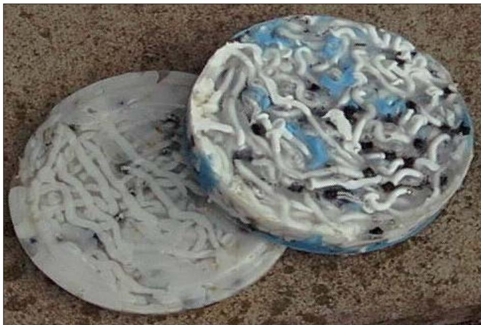
**Figure E1. "Bricks" of approximately 100 melted needle-syringes produced by the Demolizer™ melter device. Needles are embedded safely within the brick (photograph courtesy: Anthony Battersby).**
