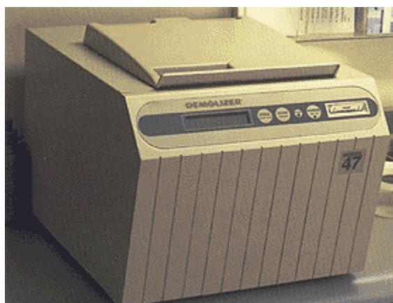
**Figure E2. The table top Demolizer™ device which heats needle-syringes until they melt and then cool into a solid piece. (UNIVEC, Farmingdale, NY, [www.univec.com](http://www.univec.com))**
