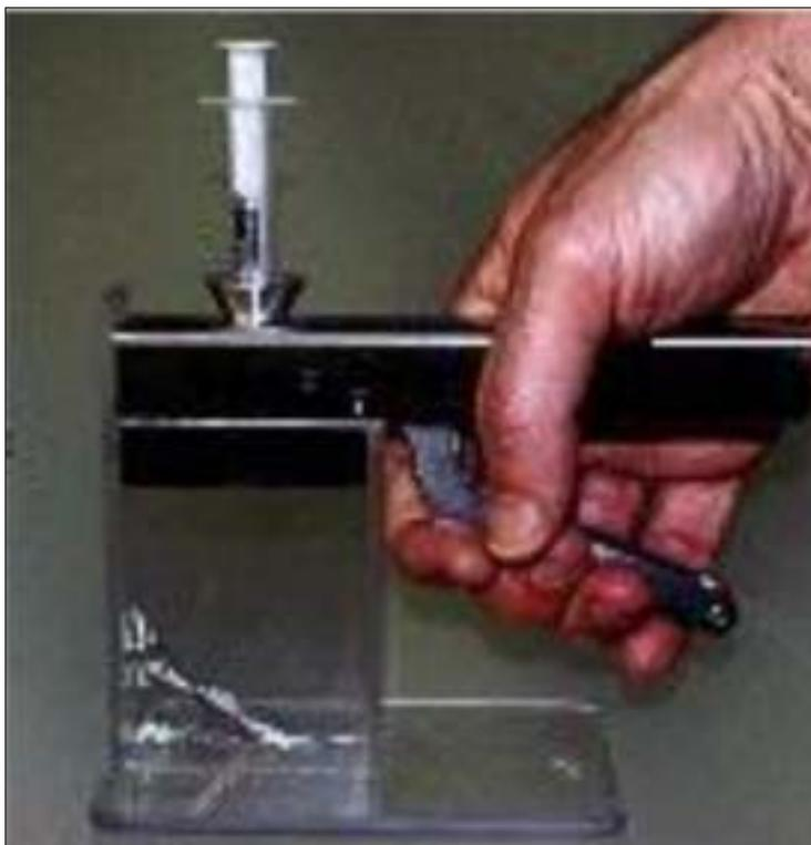
**Figure E7. Prototype PATH needle defanger with rectangular clear plastic needle container and table base**
