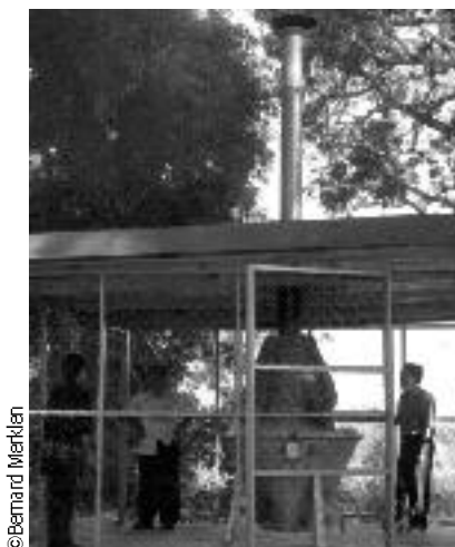
A Sicim incinerator, the type widely used in Cambodia for syringe disposal
